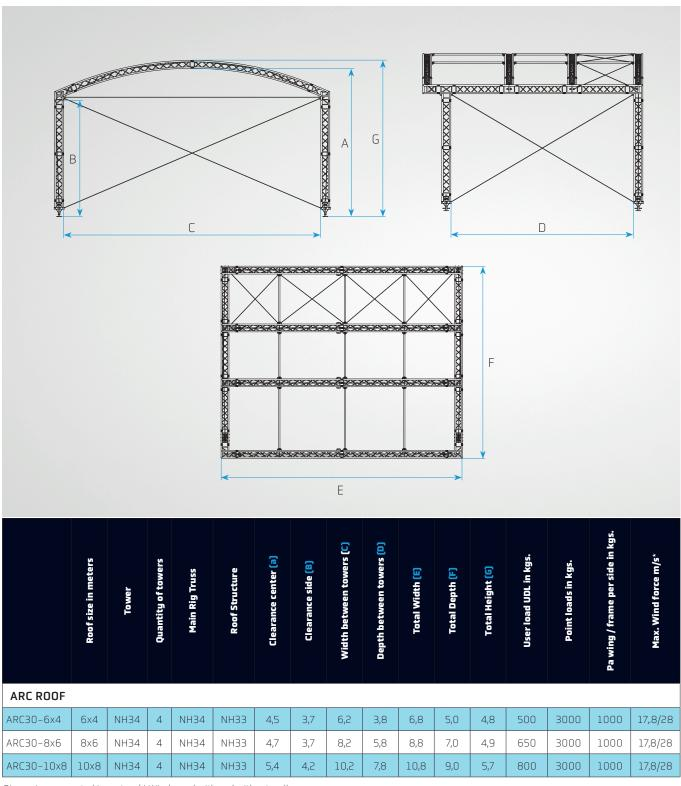
Dimensions are noted in meters |\* Windspeed with and without walls
