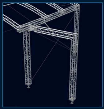
For the ARC30 roof PA Wings are available and extend the width of the ARC roof by 3 meters on each side. The PA Wing itself is 2 meters in width. The maximum load is 1.000 kg CPL on each side.
