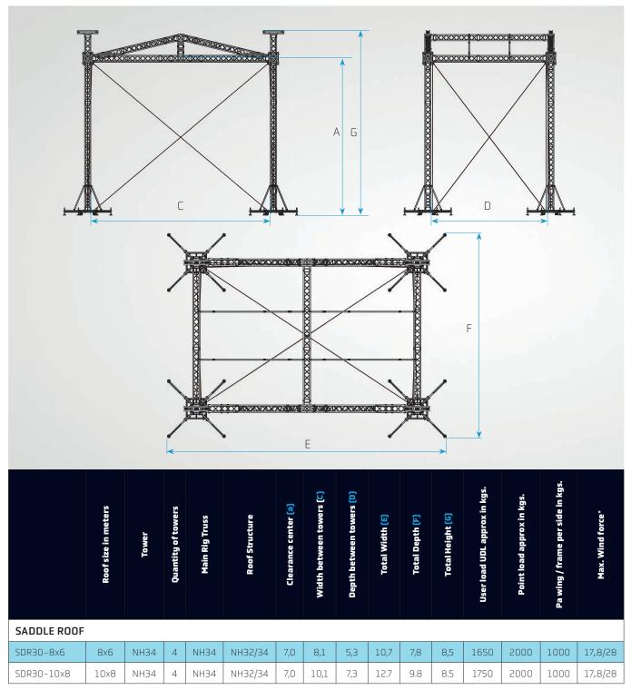
Dimensions are noted in meters | \* Windspeed with and without walls
